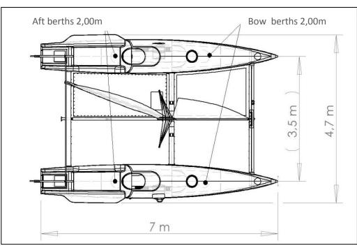
Sport Version of catamaran *Nawiatr N700K* is made in vaccum techniques out of glass, epoxy resin and core material Herex. Due to the technology and materials weight of Sport version does not exceed 550kg with less then 130kg of single hull. Standard version is 100kg heavier.
